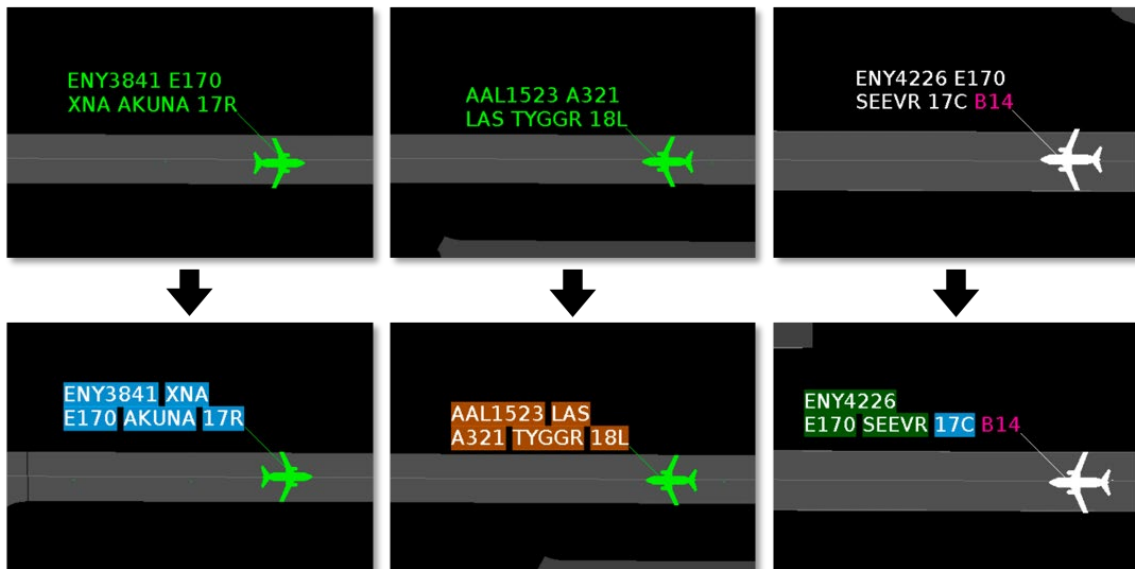
Figure 4.59. Extended Datablock Configuration: Default (top) and Ramp (bottom). Left: Departure assigned to an east-side runway. Middle: Departure assigned to a west-side runway. Right: Arrival that landed on an east-side runway.
