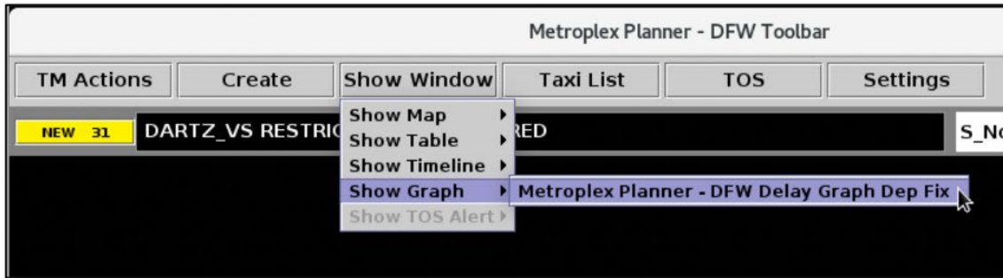
Figure 3.214. Toolbar: Show Window. Choose an existing Map, Table, Timeline, Graph, or TOS Alert window to bring it to the front of the display.
