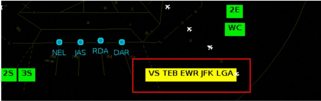
Figure 3.175. TOS Route Availability Labels on the Map. Click on a yellow label to view restrictions.
