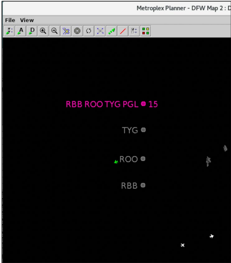
Figure 4.81. Map Labels: Closed departure fixes are grayed-out and MIT restrictions are indicated next to the fix label.
