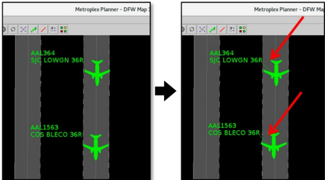
Figure 4.10. Use a keyboard shortcut to toggle between leader lines hidden (left) and leader lines displayed (right).
