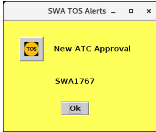
Figure 3.234. TOS Visual Alert in Flight Operator versions of the Metroplex Planner: ATC has approved a TOS reroute.
