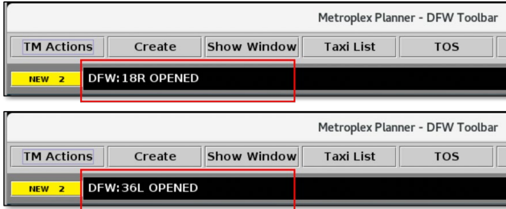
Figure 3.101. Runway closure expiration/cancellation is indicated in the Notification Banner. In this example, runway 18R/36L is reopened.
