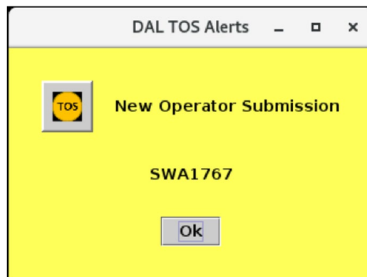
Figure 3.232. TOS Visual Alert in ATC versions of the Metroplex Planner: Flight Operator has submitted a flight for TOS rerouting.
