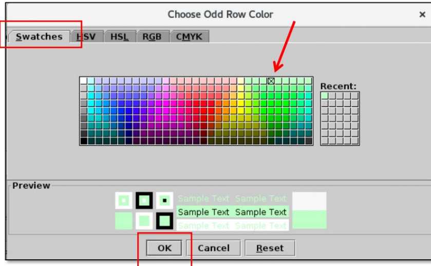
Figure 3.109. Use the “Swatches” tab to select a color. Use the HSV, HSL, RGB, or CMYK color palettes to refine the color selection, if necessary.
