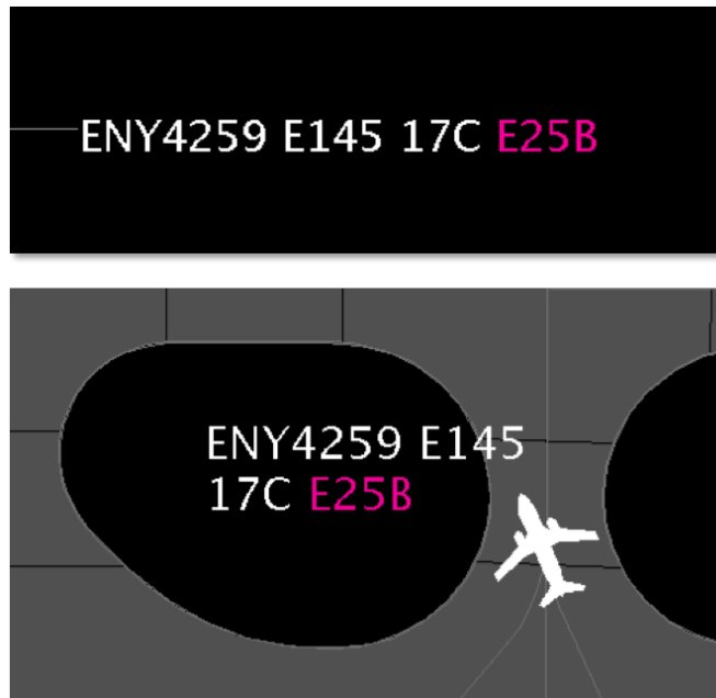
Figure 3.236. Gate Conflicts: In this example, Gate E25B is occupied, as indicated by the magenta gate number in the arrival flight's datablock on the timeline (top) and map (bottom).
