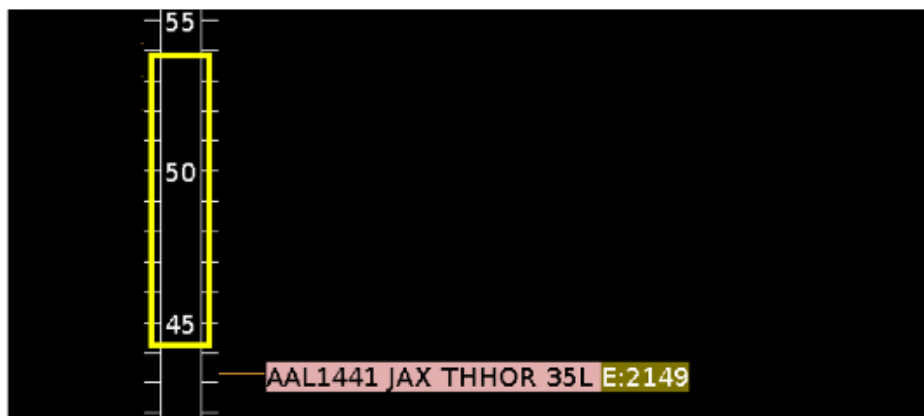
Figure 6.50. EDCT compliance on the Timeline. Yellow highlight: Flight is predicted to be released from the runway earlier than its -5/+5 min EDCT compliance window.
