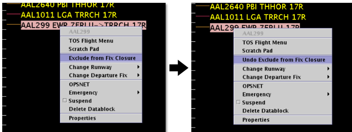
Figure 7.2. Right-click Menu: Exclude from Fix Closure (left), Undo Exclude from Fix Closure (right).
