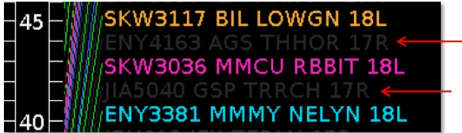
Figure 6.46. Datablocks of flights in a deselected category are grayed-out on the timeline.
