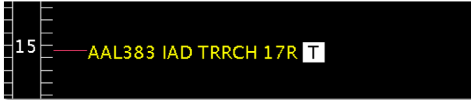
Figure 5.71. On the timeline, a “T” highlighted in white indicates that the Flight Operator has submitted one or more TOS routes for that flight.
