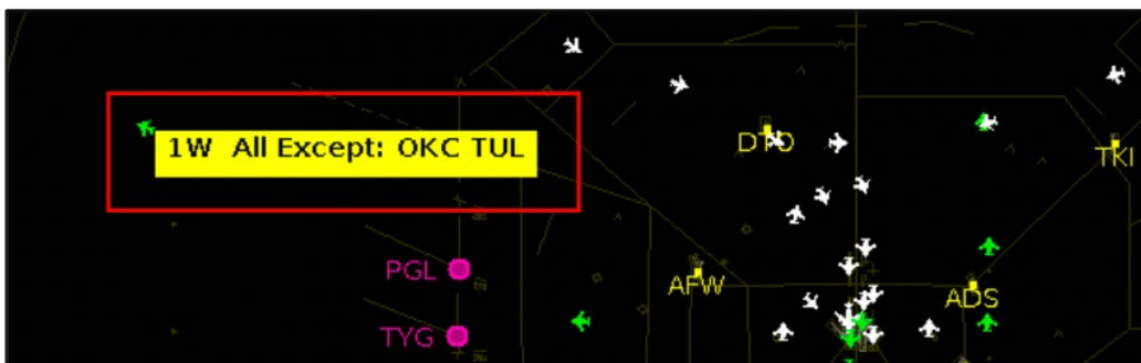
Figure 3.202. TOS Route Availability Labels on the Map. In this example, the PGLET “1W” CDR is color-coded yellow because it is closed except for OKC- and TUL-bound flights.
