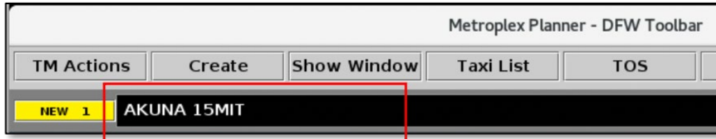
Figure 3.18. MIT restriction in the Notification Banner. In this example, there is a 15 MIT restriction on the AKUNA departure fix.
