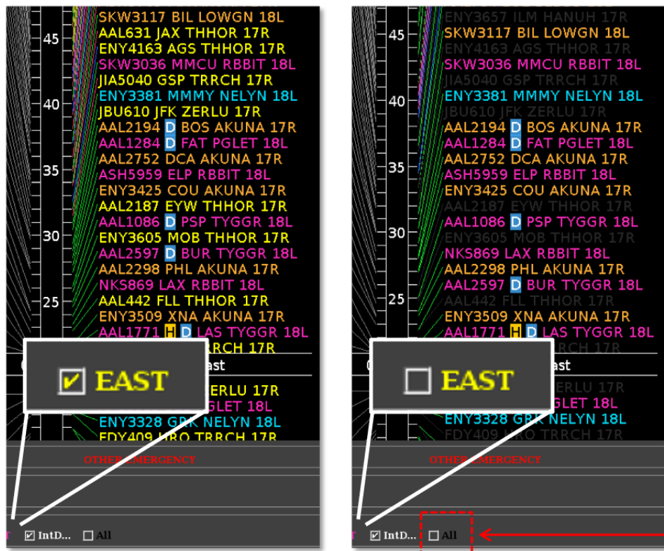
Figure 6.45. Deselect a category in the Timeline legend. In this example (right), the “East” departure gate is deselected. As a result, those datablocks are grayed-out on the timeline (right).
